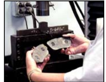
Our engineers conduct shear testing on Raybestos and competitive disc pads. This test measures the amount of force required to "break off" the friction material from the steel backing plate.
